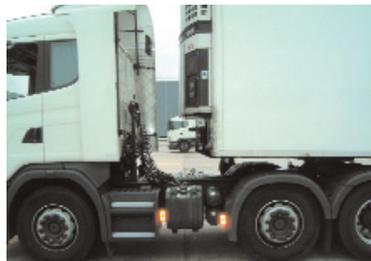
The first stage of the procedure involves the connection of the trailer to the 5th wheel whilst it is located rearward of the normal
