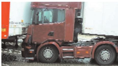
The roll away of a trailer, when the towing unit is correctly parked, is likely to have the same consequences as a complete vehicle or towing unit run away. In many cases the cause of this type of accident is due to bad practice of both the driver who left the trailer without applying the parking brake, and the driver coupling to the trailer, who did not check that the parking brake was applied and subsequently has the accident.
