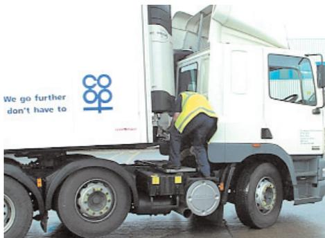
The procedures in annexes 2 and 3 provide a means of coupling and uncoupling close coupled combinations and should be followed whenever a safer method cannot be used. These methods are not intended to be a substitute for applications that allow the use of the standard procedure detailed in annex 1 on a close coupled combination.
