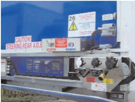
operational conditions, it was not universally possible to overcome the problems encountered whilst connecting the air and electrical services on close coupled semi trailers. However, moveable arms may be a solution to the coupling and uncoupling problems encountered on some types of vehicle combination, and may be used where a 'Risk Assessment' indicates it to be appropriate.
